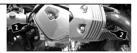
3. Insert bottom tab of the X-head tab between lower spark plug cover and cylinder head. Install the 16mm M6 hex bolt (washer is not needed) and secure tab with 5mm hex wrench.
