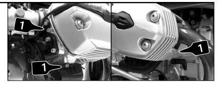
2. Screw in aluminum spacers by hand and lightly snug down with a 13mm wrench. **DO NOT OVERTIGHTEN.** Overtightening may cause the shank of the spacer to break.
